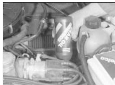
27.4b . . . then top up via the breather/filler plug orifice
