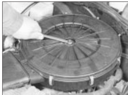
24.1a On carburettor models, undo the retaining nut (on some models the lid will be retained by screws) . . .
